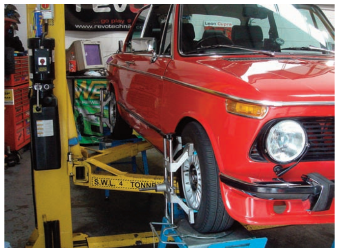
Have the suspension geometry checked and adjusted by laser alignment
