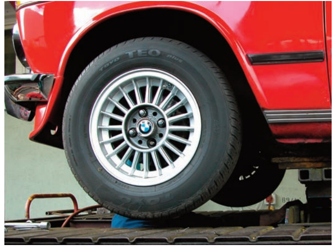
Adjust the ride height to approximately the mid way position as a starting point
