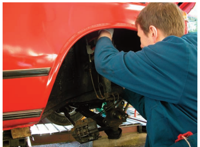
Fit spring compressors and compress the spring
