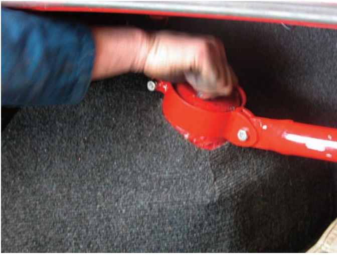
and unbolt the dampers from the turrets inside the boot.
