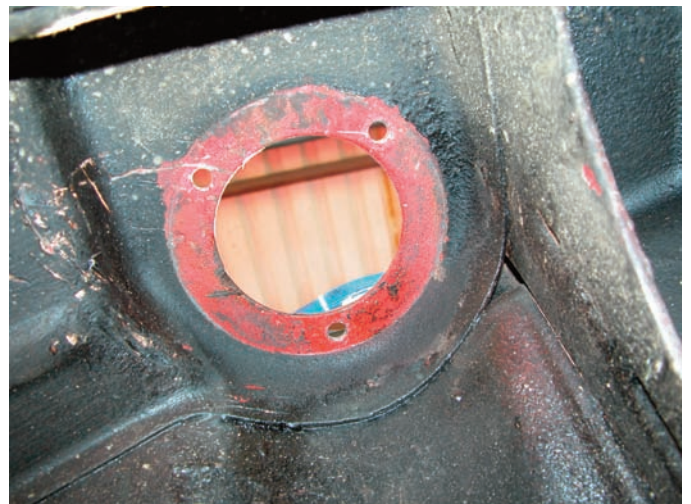
Now's a good time to check the condition of the suspension mounting position on the inner wings. This one still has the original paint showing after 37 years!
