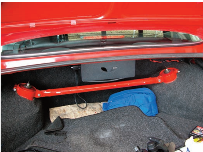
A rear strut brace is recommended to reinforce the rear turrets when coilover suspension is used
