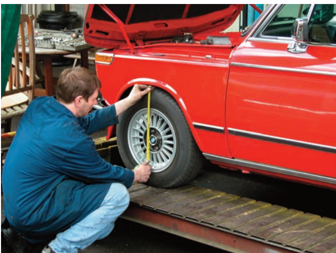
Check side to side ride height and adjust as required. Test drive and check for knocking or scraping. Adjust as required.
