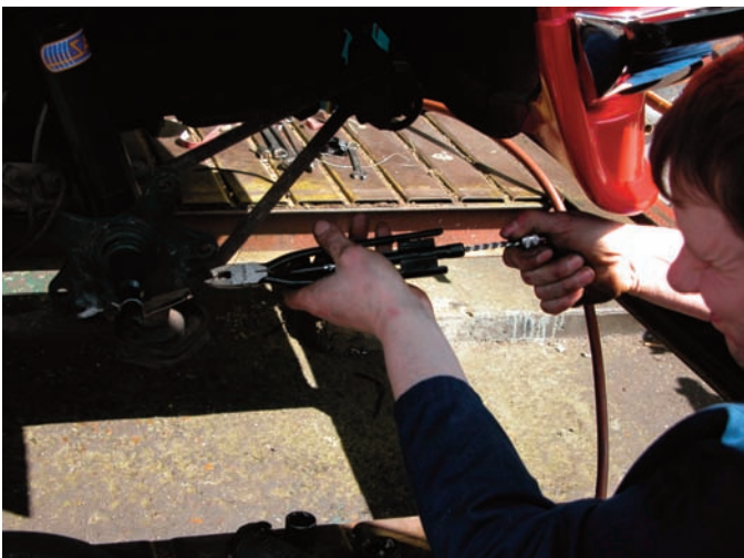
... and secure with stainless steel locking wire. The lock-wire pliers grip the two ends of the wire; the jaws are locked and the knob is pulled to spin the pliers and twist the two ends tightly together
