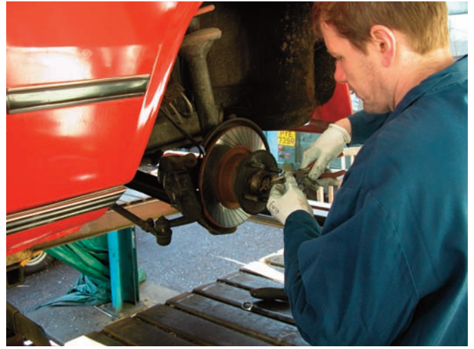
Disconnect the brake hose bracket and caliper from the strut and tie it out of the way by fixing the caliper on to the track rod with a length of wire.
