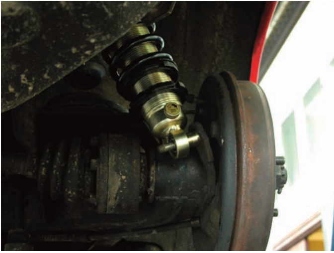
Fit the bottom end of the coilovers on to the bolt using the spacers supplied and fit the securing nut.
