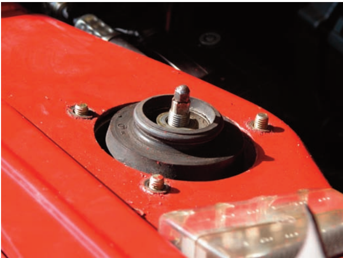
Fit washers and Nylock locking bolts
