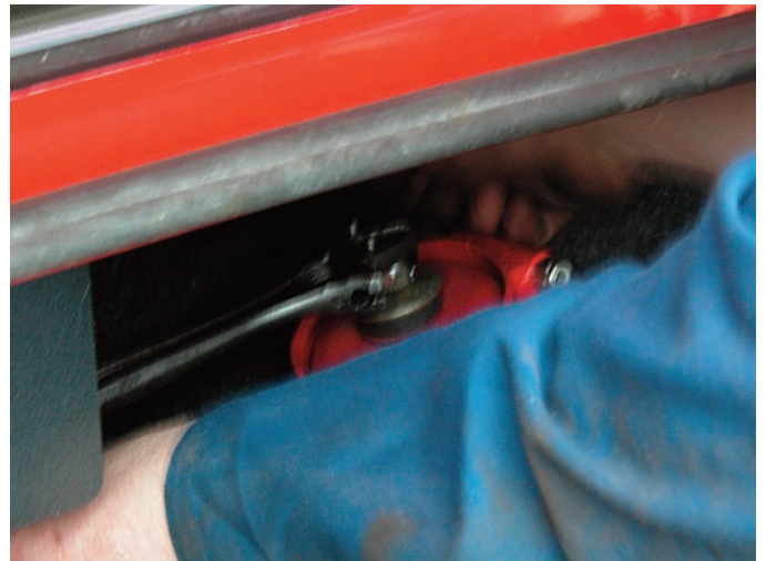
...holding the centre rod steady while turning the securing nut
