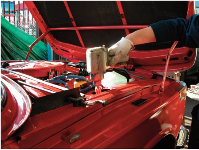
Remove central nut from strut to release the top mount
