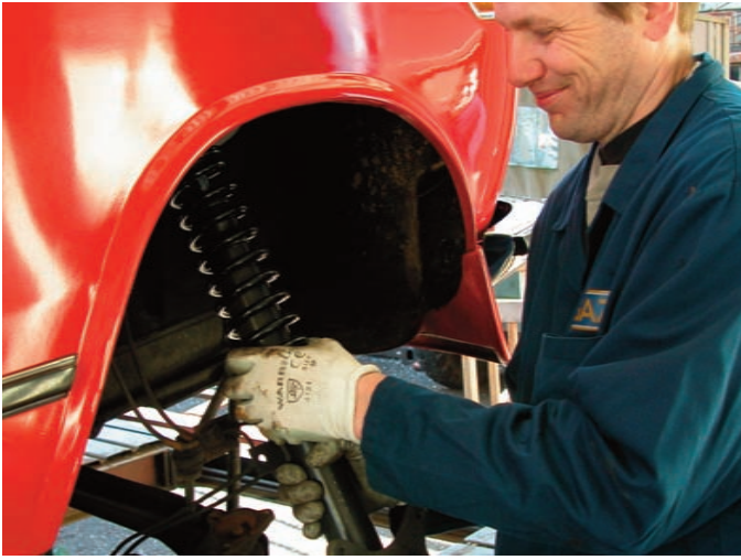
Install the coilover unit...
