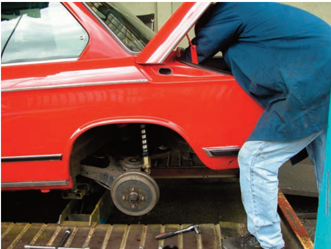
Fit the new rubbers and install the GAZ coilovers into the turrets and secure...
