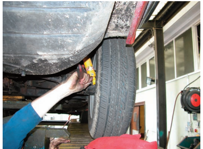
... and start work on the back by unfastening the damper lower bolts
