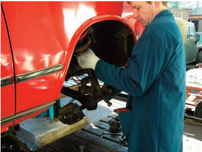
Pull the strut outward at the bottom and down to remove
