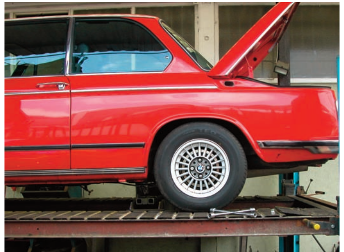
Adjust the ride height to give a very slightly nose down attitude. Check for clearance around the wheel arches
