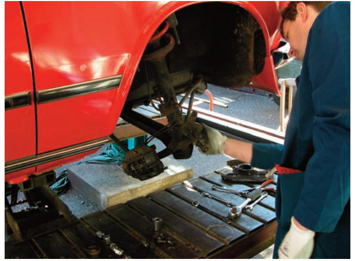
Disconnect strut lower bolts after first removing the locking wire (if present)
