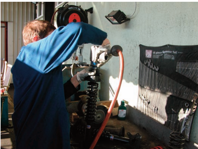
Using the height adjuster collars on the new coilover, set the coil springs to the lowest setting and secure the top mount, tightening the nut securely with an air gun
