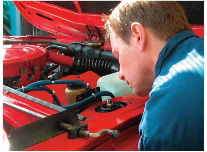
... lining up the top mount bolts with the holes in the inner wing
