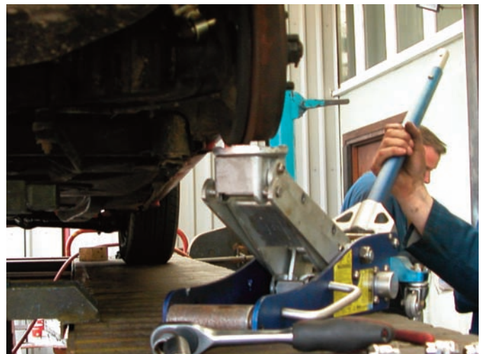
Use a trolley jack to raise the rear suspension until the coilover's bottom mount can be lined up with the mounting bolt
