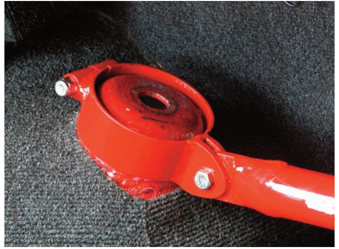
Remove the rubber mounting collar from the hole in the turret top - the GAZ unit come with new rubbers
