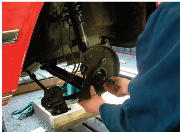
Refit the backing plate and hub (we fitted new bearings while it was off) and adjust the wheel bearing. Refit the caliper and hose bracket
