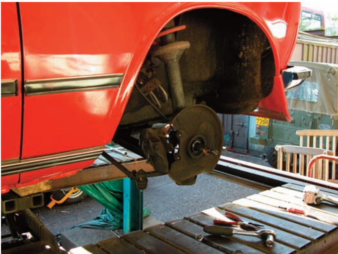
Remove the split pin and hub nut and remove the hub complete with brake disc
